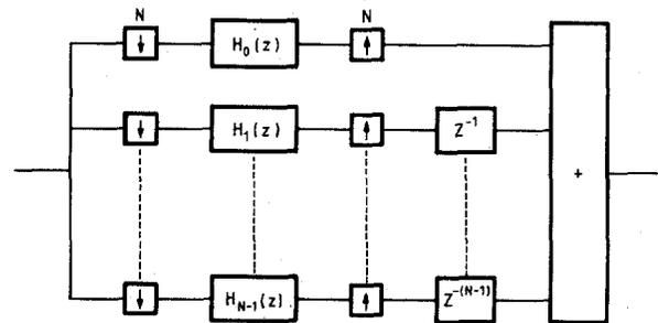
Fig. 1. Low-pass polyphase network. Arrows denote sample rate decrease and increase, respectively.
