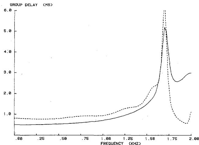
Fig. 4. Group delay of four-channel transmultiplexer filter: — = WD filter, - - - = Bellanger filter.
